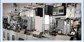
The End of Line Test station ensures correct performance of every caliper we produce.
